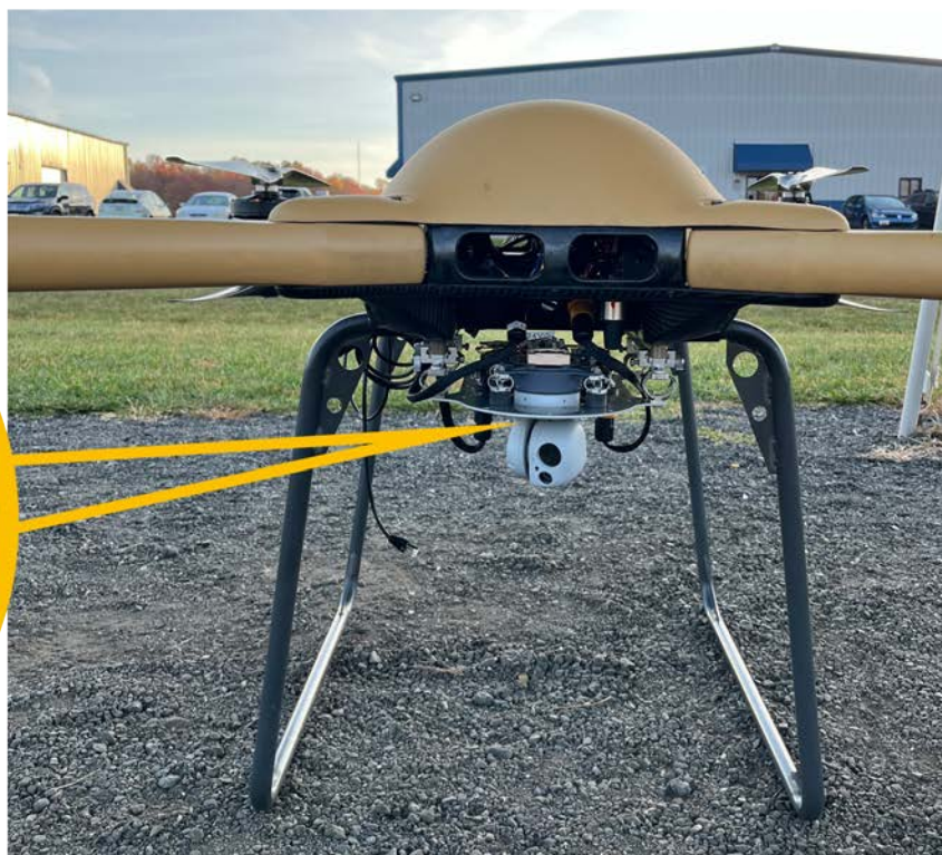
■ R2D2 mounted to the Tactical Resupply Vehicle (TRV)-150C for testing. Image courtesy of CMI2.
